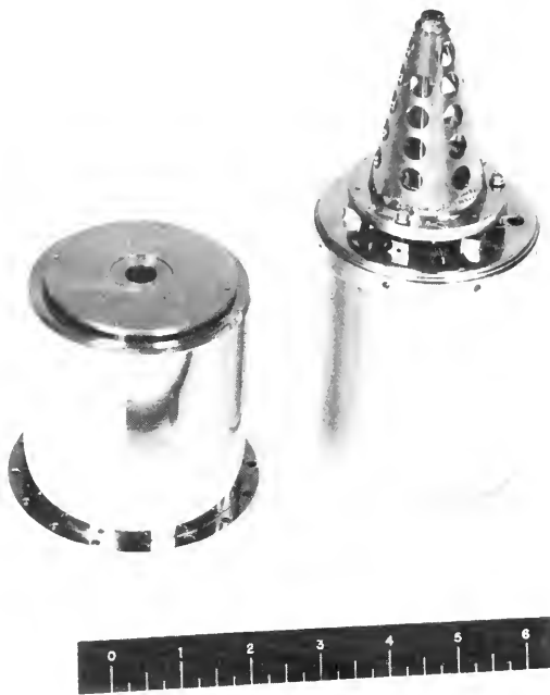
FIGURE 11-40.—The DME-A quadrupole mass spectrometer with cover removed. The analyzer section is located within the perforated cone. Scale is in inches. (Courtesy of R. Narcisi.)
